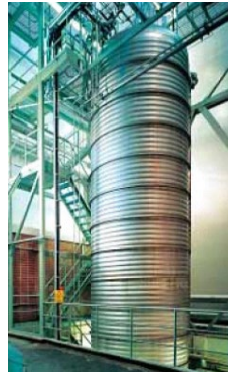
Figure 2. An industrial fermenter. Some indication of its size can be gained from the series of steps at the left of the photograph. Its diameter is about 6 m and its height about 20 m. Image from www.vaahtogroup.fi .
